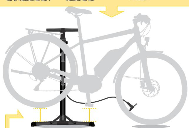
**Be aware of the distance between wheel and support legs and ensure there is no interference while operating the crank.**
