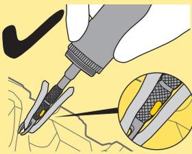
When repairing a tire puncture, avoid twisting Plug Tool to keep the inflation orifice clear. If the inflation orifice is blocked by the repair plug, CO2 gas may leak from the tool during inflation
