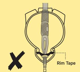
Do not insert the plug tool too deep, otherwise it may puncture the rim tape and cause an air leak
