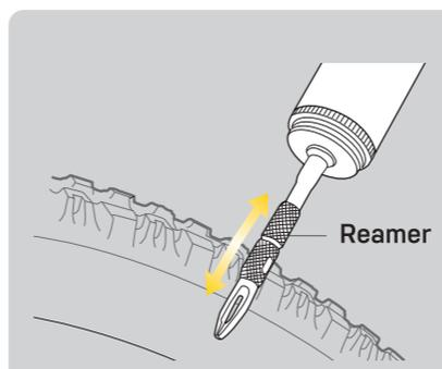
**Use the Reamer to roughen the area around the hole before repair**
