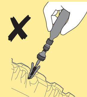
To prevent accidental discharge, do not repair tire puncture while an unused CO2 cartridge is mounted in the CO2 inflator
