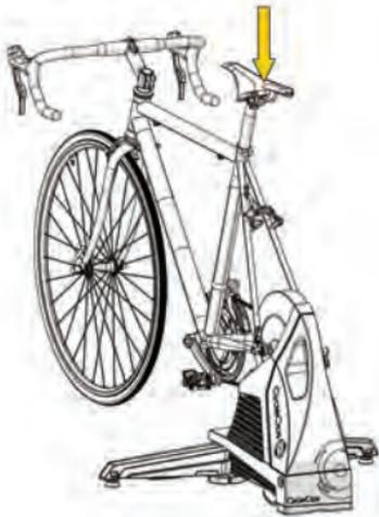
**EN** Press the saddle down and lift the front wheel from the ground to confirm that the frame has been completely fixed to the trainer.
